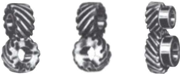
TWO RIGHT-HAND HELICAL GEARS
