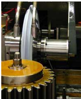
Gear Grinding using a Single Rib Wheel
